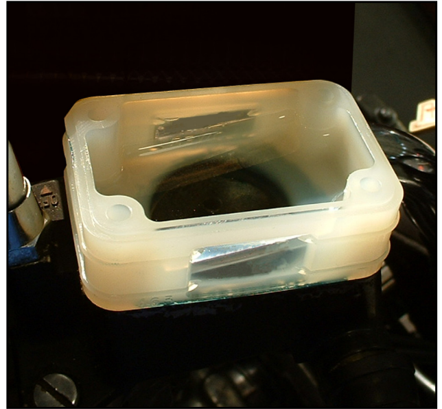
Machined carriage made of LDPE
